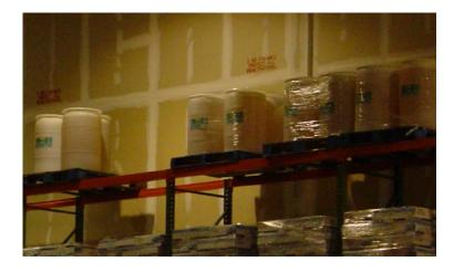
C) Unused pallets were stacked and stored in a manner that blocked the most direct route to a fire exit from the end of an The pallets were stacked about 15 feet There is high. no designated overflow location in the warehouse for pallets or other goods.
